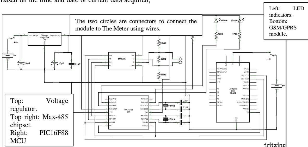
**Figure 1:** Circuit diagram of the module.
