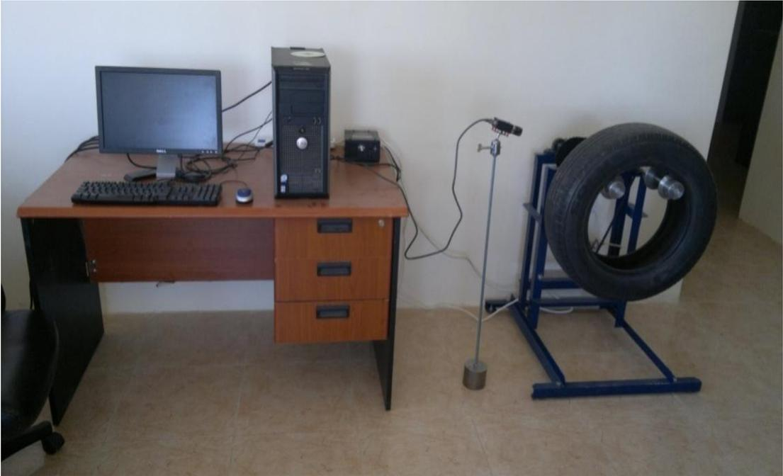
Figure 5: The entire system used for taking samples which contains pc, linear camera and rotating machine
