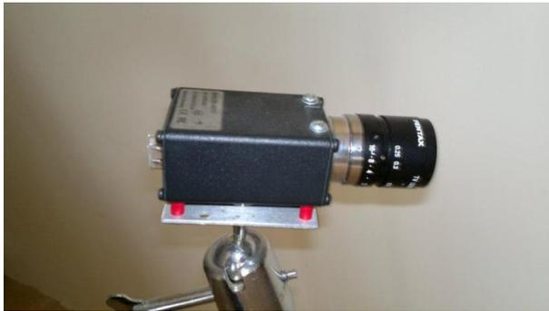
**Figure 2:** Basler linear camera used for taking samples of tires
