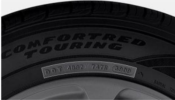
**Figure 1:** DOT code region on tire sidewall image
