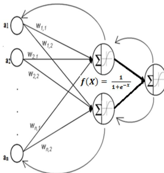
**Figure 1: Back-Propagation Multi-Layer Neural Network**
