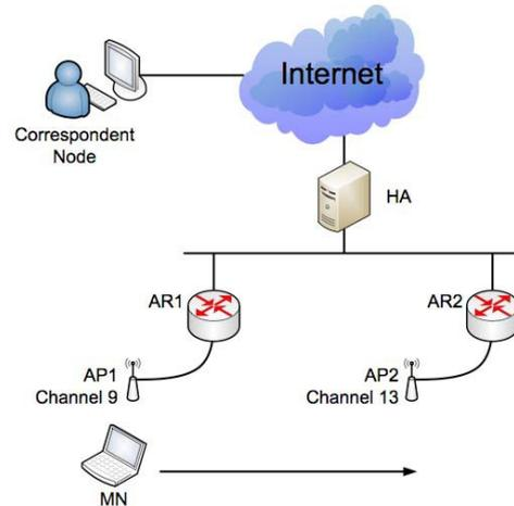
**Figure 7:** Testbed used in the experiments
