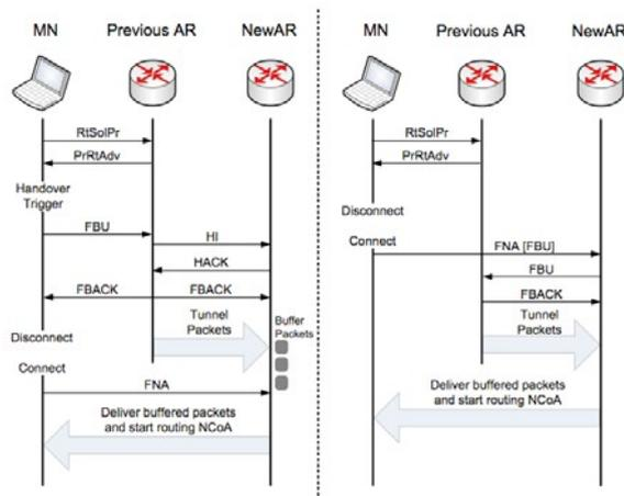
**Figure 3:** FMIPv6 protocol operation: Predictive mode (left) and Reactive mode (right)
