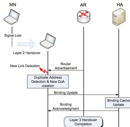
**Figure 2:** Layer 3 handover managed by the MIPv6 protocol
