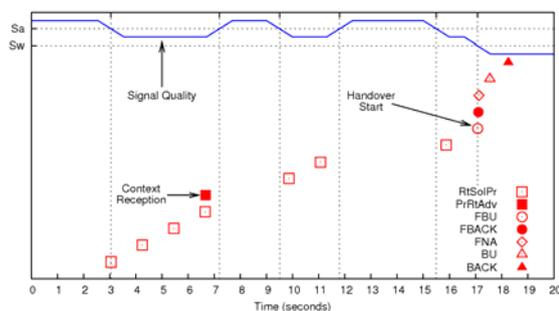
**Figure 8:** Candidate access points discovery followed by an FMIPv6 predictive handover
