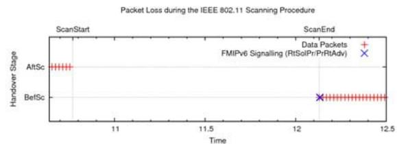
**Figure 4:** Packet loss and latency during a scanning for discovery of candidate access points
