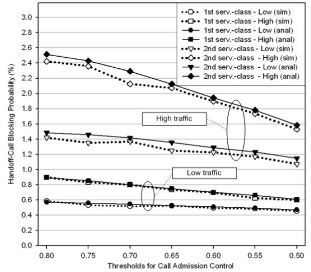
**Figure 5:** Handoff-call blocking probabilities vs new-call admission control thresholds (quasi-random traffic).
