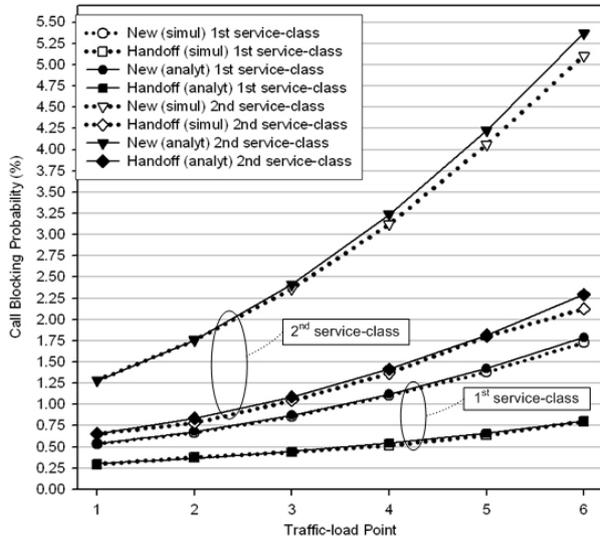
**Figure 4:** New-call and handoff-call blocking probabilities vs offered traffic-load (quasi-random traffic).
