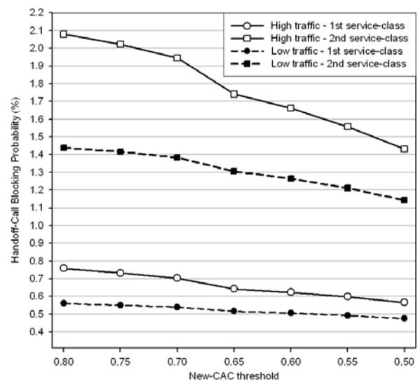
**Figure 3:** Handoff-call blocking probabilities vs new-call admission control thresholds (Poisson traffic).
