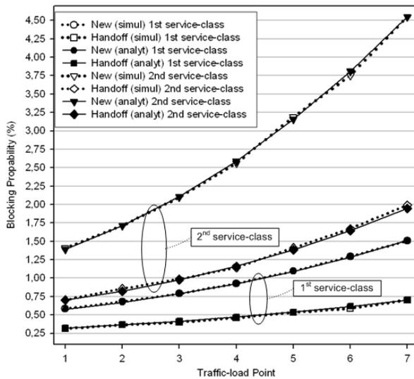
**Figure 2:** New-call and handoff-call blocking probabilities vs offered traffic-load (Poisson traffic).
