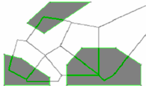
Fig. 4. Voronoi Diagram of the obstacle corners
