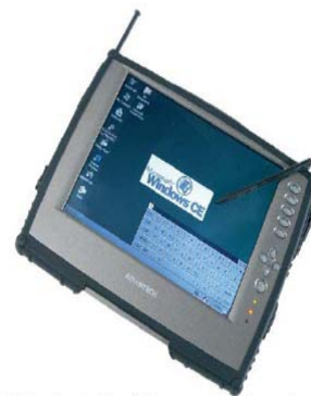
Figure 15. Tablet PC equipped with wireless communication used as a mobile control and supervision center. (Courtesy of Setex and Advantech)
